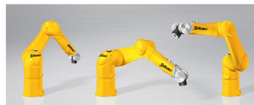
TX2-90 6-axis industrial robot
